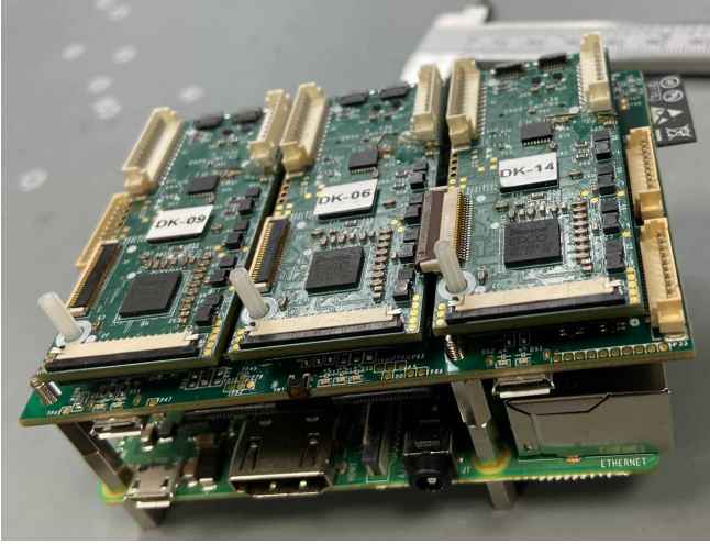
Figure 4: DAVID Platform – Hub with 3 Inference node daughter boards fully assembled for placement in a smart-toy.
